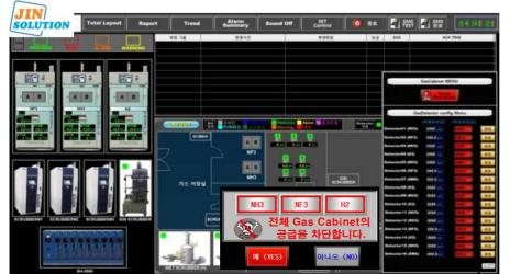
This system can check the status of the gas supply system in real time in the control room or office, and manage the history and prevent safety accidents through the operation status check and remote control of each supply system.
